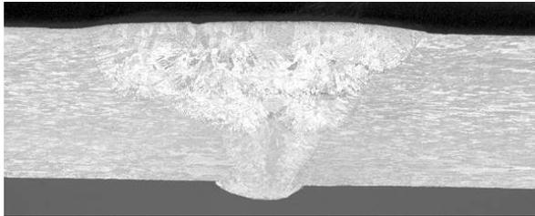
Manual plasma welding provides defect-free welds of a required thickness.
