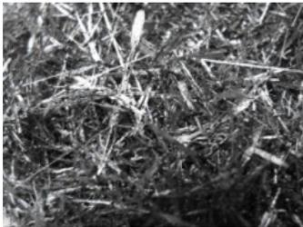
In addition, during the experiments were obtained filiform spraying products (accepted definition is a needle or tube). Obtained powders are suitable for use in the chemical industry as fillers for filters
